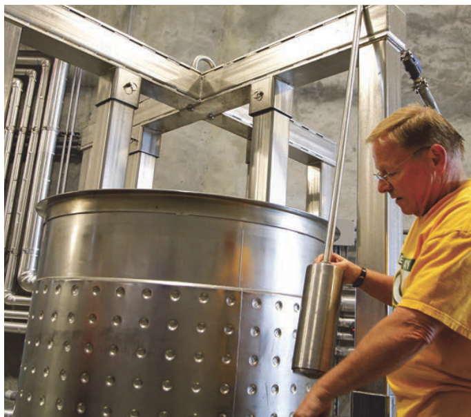
Winemaker TJ Rodgers discusses the wine press he designed. The press moves between utility stations in the fermentation cave, pressing each tank in as little as 25 minutes.
