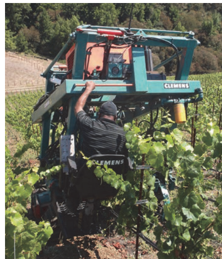
Clemens GmbH helped TJ Rodgers create an over-the-row tractor guided by cables that can handle the steep vertical and horizontal slopes at the Domaine Lois Louise vineyard.
