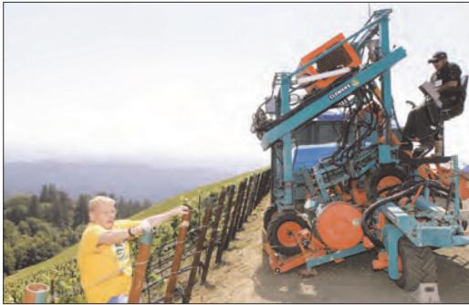
T.J. Rodgers invented a tractor that can traverse a 35-degree slope for his winery.
